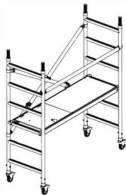
Base Unit Width: 680mm Length: 1910mm Height: 2082mm
