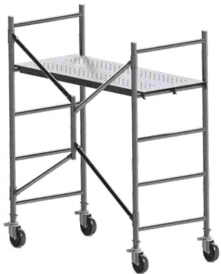
5ft Aluminum X Type Folding Scaffold ERP #:14220500030 Material:Aluminum 6061-T6 Size(mm):1250X600X1524 Weight:24.4kg Safe Working Load:200kg
