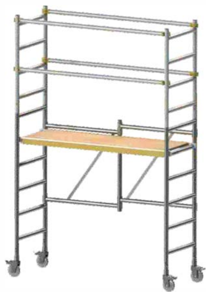
Aluminum Z Type Folding Scaffold w/Guardrail System ERP #: AFS-Z-28 Material: Aluminum 6061-T6 Size(mm): 1910X680X2830 Weight: 47.3kg Safe Working Load: 150kg
