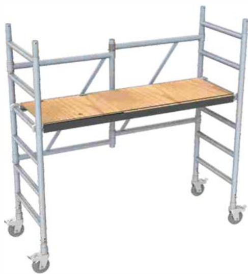
Aluminum Z Type Folding Scaffold w/o Guardrail System ERP #: AFS-Z-18 Material: Aluminum 6061-T6 Size(mm): 1910X680X1803 Weight: 36.9kg Safe Working Load: 150kg
