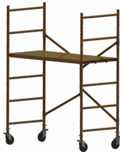
6ft Steel X Type Folding Scaffold ERP #:14220600023 Material:Steel Q235 Size(mm):1400X700X1727 Weight:53.8kg Safe Working Load:280kg
