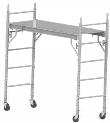
Aluminum Multifunctional Scaffold Guardrail System can be optional subject to your specific working demands. ERP #: AMS16 Material: Aluminum 6061-T6 Size(mm): 1833X695X1651 Weight: 38.4kg Safe Working Load: 450kg
