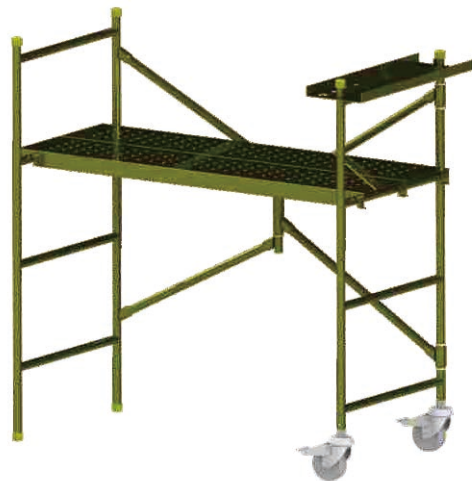
4ft Steel X Type Folding Scaffold w/ single side wheels ERP #:14220400033 Material:Steel Q235 Size(mm):1168X533X1220 Weight:32.9kg Safe Working Load:150kg
