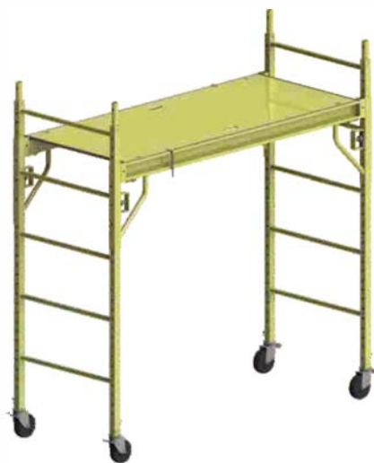
Steel Multifunctional Scaffold Guardrail System can be optional subject to your specific working demands. ERP #: SMS16 Material: Steel Q235 Size(mm): 1828X698X1651 Weight: 66.1kg Safe Working Load: 450kg
