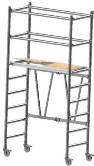
Aluminum V Type Folding Scaffold w/ Guardrail System ERP #: AFS-V-28 Material: Aluminum 6061-T6 Size(mm): 1400X680X2852 Weight: 49.6kg Safe Working Load: 150kg
