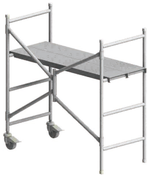
4ft Aluminum X Type Folding Scaffold w/ single side wheels ERP #:14240400020 Material:Aluminum 6061-T6 Size(mm):1168X533X1222 Weight:14.6kg Safe Working Load:150kg
