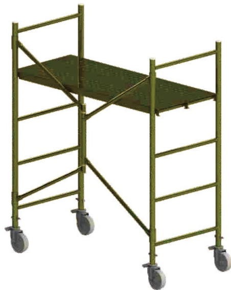
5ft Steel X Type Folding Scaffold ERP #:14220500013 Material:Steel Q235 Size(mm):1250X600X1524 Weight:25.7kg Safe Working Load:200kg
